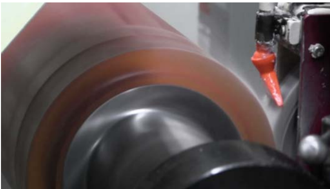
Roll being ground with coolant
